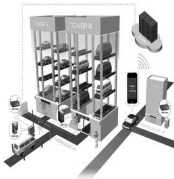
Figure 2. Multi-level car parking system
